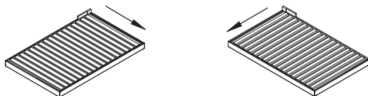
Construction type 4: Fitted on an open construction (No mounting holes) Liberty
